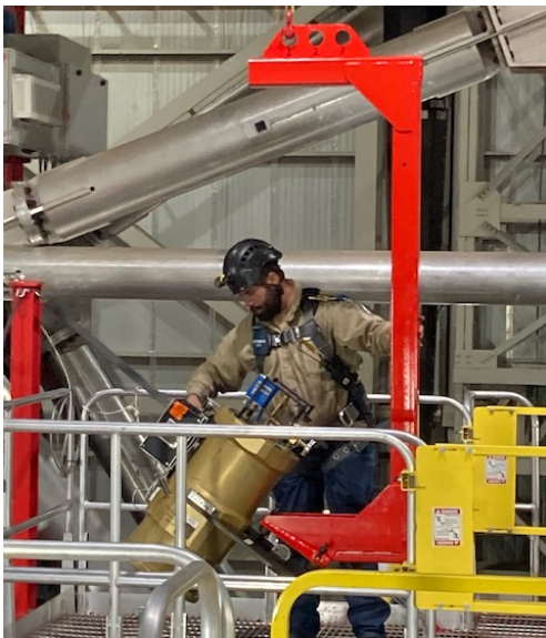
Installation of the dewar for the SHARK-NIR scientific camera, with assistance from LBTO staff member Tim Castro.
